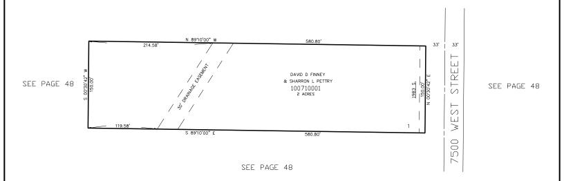
10' UTILITY & DRAINAGE EASEMENTS EACH SIDE OF PROPERTY LINES AS INDICATED BY DASHED LINES EXCEPT AS OTHERWISE SHOWN.
